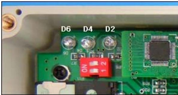
On the GSM-CTL-AC board, there is one Red DIP switch, that is used to setup the relay working method. We have two way to control the relay. SMS or phone calling. You have to select one right way as your relay working way.
